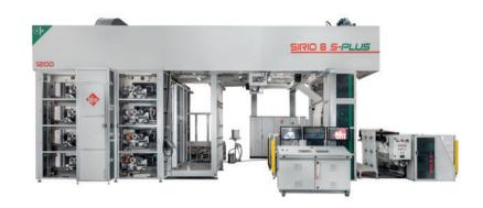
Stack type machines, designed for printing on different plastic materials for the packaging market but also Stack type 8 colours suitable for paper materials, in line with the extruder or from reel to reel. The printing repeat length is from of Italy, bfm srl delivers two more 350 mm up to a maximum of 1200mm,
