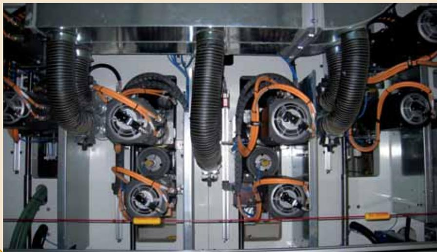
Bosch Rexroth's leadership in providing solutions for the printing industry is confirmed by the number of motors certified for use in potentially explosive areas: the MKE series, which is part of the IndraDyn S brushless motor range, is the version that can be mechanically interchanged with the standard MSK range.
